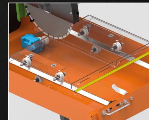
Working table sliding on 6 nylon wheels: in top 4 pulleys with 8 ball bearings; below 2 pulleys on 4 bushes in stainless steel. Higher precision and stability
